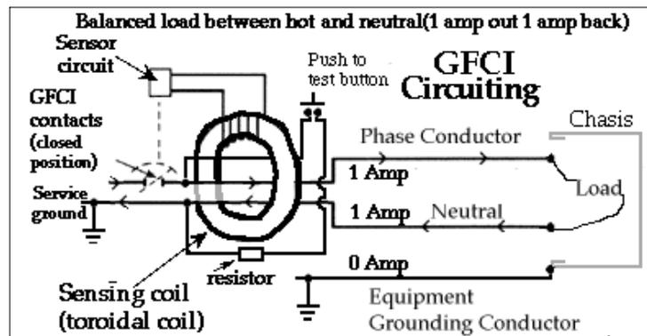
The GFCI will trip in a fraction of a second at currents (a few mA) well below those that are considered dangerous. Note that a GFCI is NOT a substitute for a fuse or circuit breaker as these devices are still required to protect equipment and property from overloads or short circuits that can result in fire or other damage.
